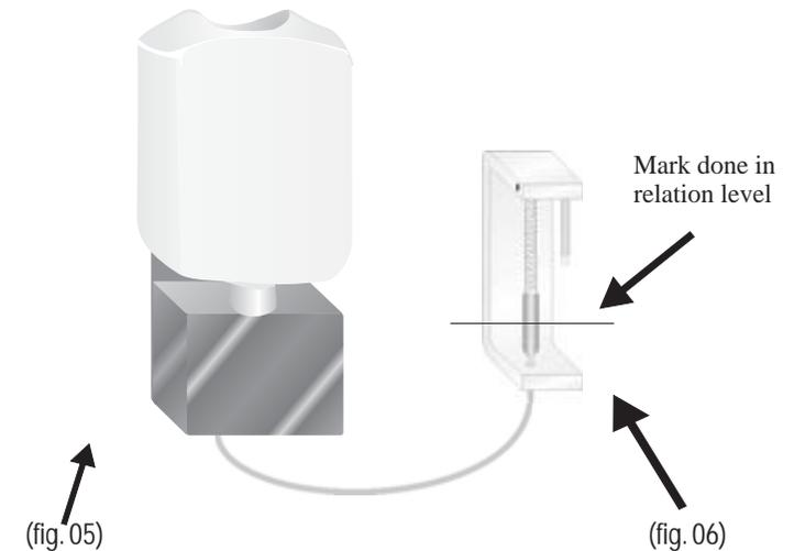
7. Connect the silica hose in the probe. Observes that the tip of cotton cord is in contact with water and that does not lack water in the plastic container.
