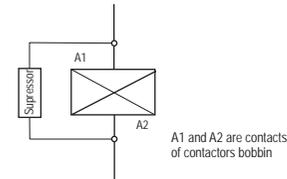
Diagram of suppressors input in loads of direct drive
