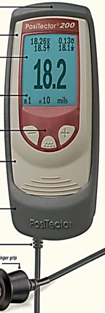
Measure paint, varnish, lacquer, etc. on wood products including cabinetry, furniture, flooring, windows and more.
