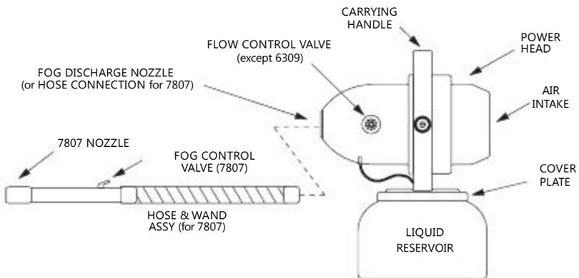
This machine has a one-gallon [4 liter] reservoir to hold fogging liquid. On the 7807 the fogging nozzle is at the end of the hose/wand assembly; on other models Except for the 7807, it is mounted in the power head;
